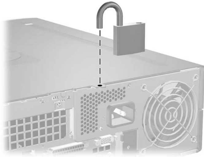
Figure C-2 Installing a Padlock
